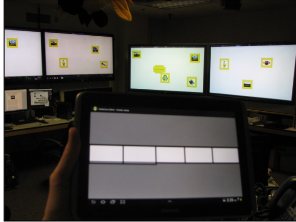
Figure 31: An example of a screen jump view. At this point the user can click on any of the white rectangles that represent wall displays and the users handheld will be jumped to that display.
