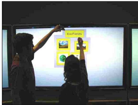
Figure 19: Reaching the top or bottom of a shared display with a finger/pen input can be difficult for users.
